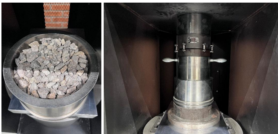
Figure 11. Photo of the test cylinder with sample prepared (left) and during loading in the Instron 400RD (right).
