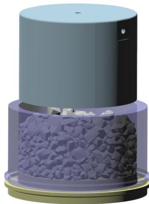
Figure 16: The oedometer rig consists of a cylindrical shell (purple), plug at the bottom (yellow) and a piston (blue). The oedometer is filled with a particle bed (grey).
