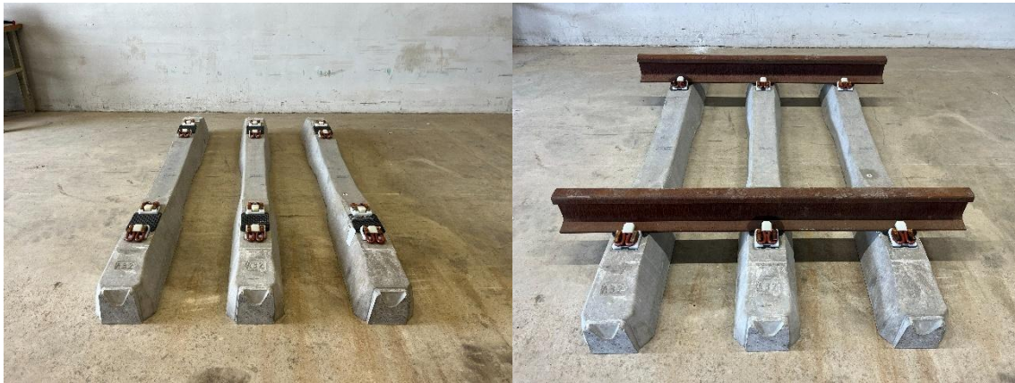
Figure 6. Left: Picture of A32 sleepers. Right: Section with mounted 60E1 rail and fasteners.
