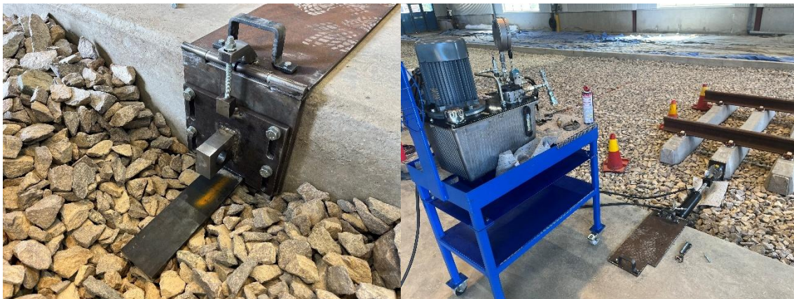
Figure 7. Left: The developed assembly to hold and align the hydraulic cylinder. Right: complete system setup with hydraulic system and sensors.
